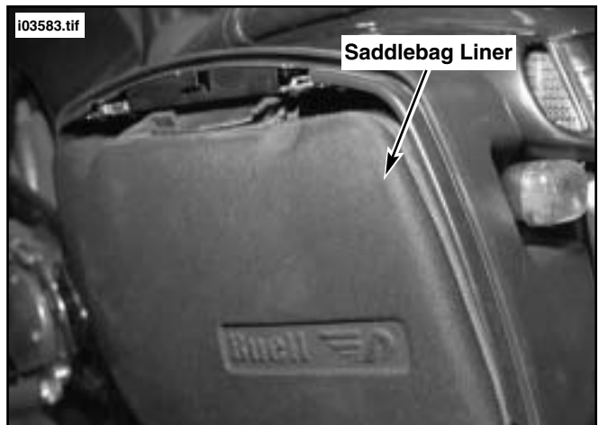
Figure 14. Install Saddlebag Liner
